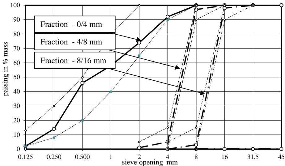
Figure 1. Aggregate grain size distribution
