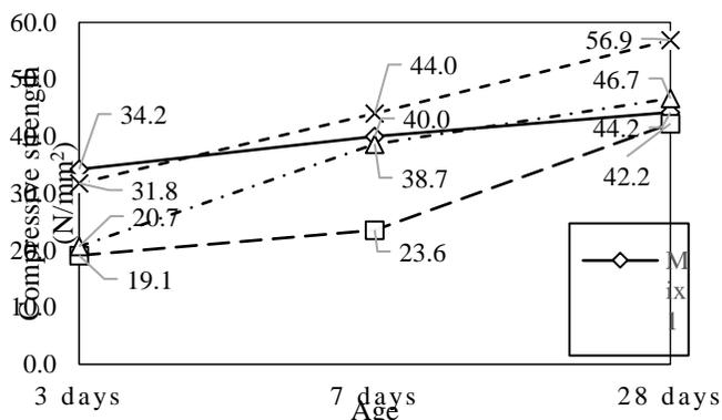
Figure 3. Compressive strength at the age of 3, 7 and 28 days
