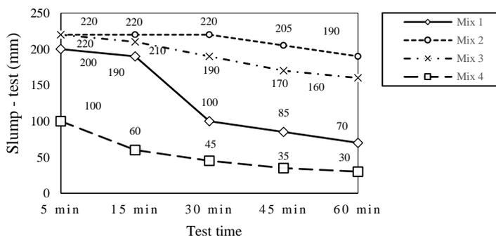
Figure 3. Slump – test in time
