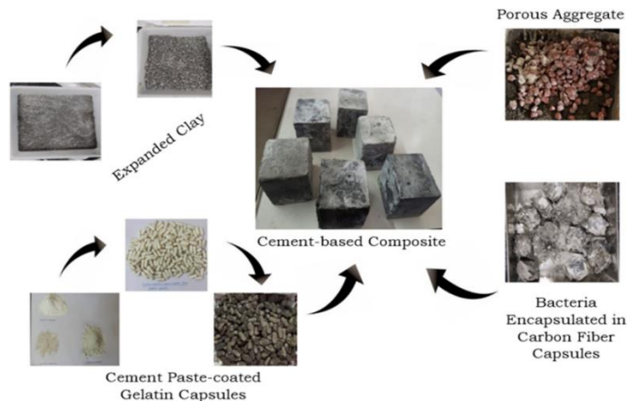
Figure 3: Immobilizing bacteria in expanded clay and porous aggregate, cement paste-coated gelatin capsules, and encapsulating bacteria in carbon fiber capsules for producing CBC samples [18].
