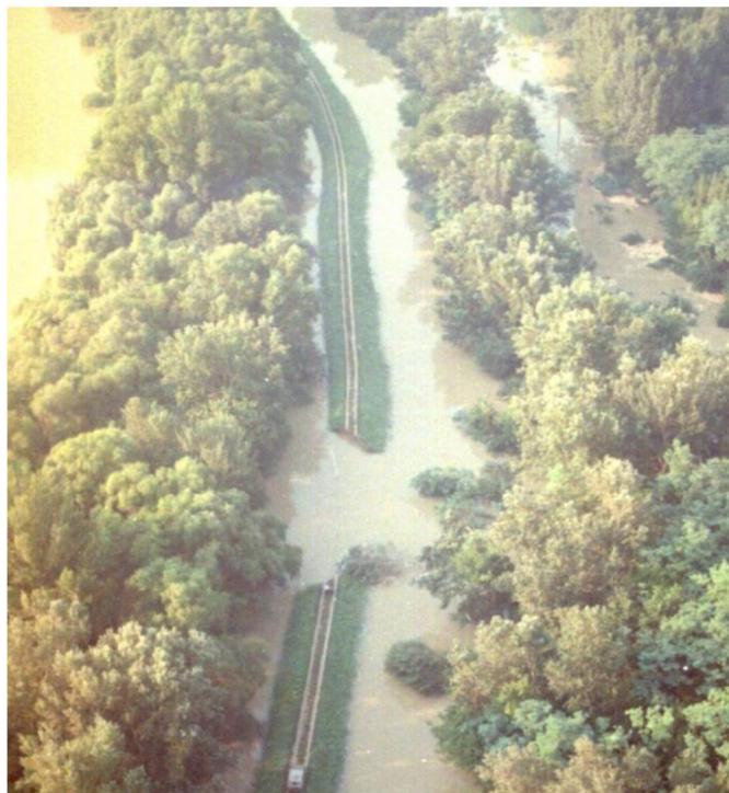
Photo 2 Dike failure at Surány city in 1991 Danube flood
