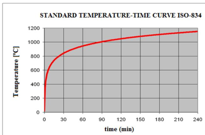
Figure 1. Standard Temperature-Time Curve ISO-834 [4]
