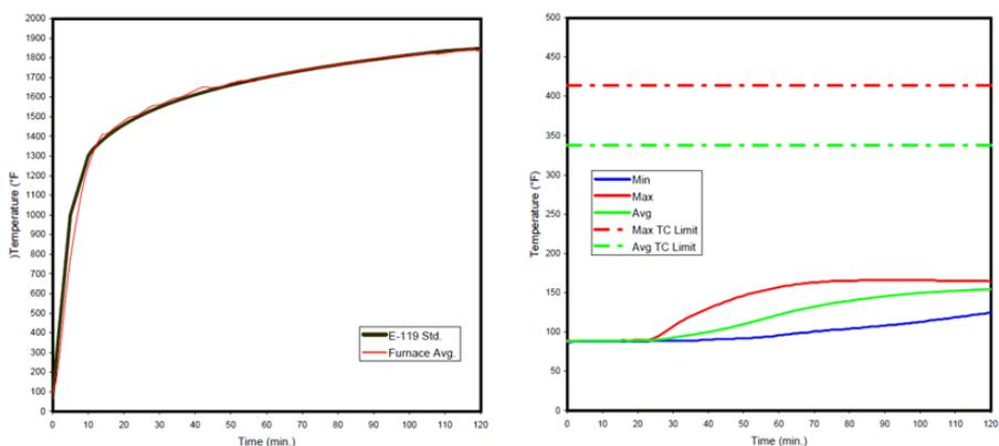
Figure 5. Furnace interior temperatures (left diagram) and minimal, average and maximal cold side temperatures (right diagram) [9]
