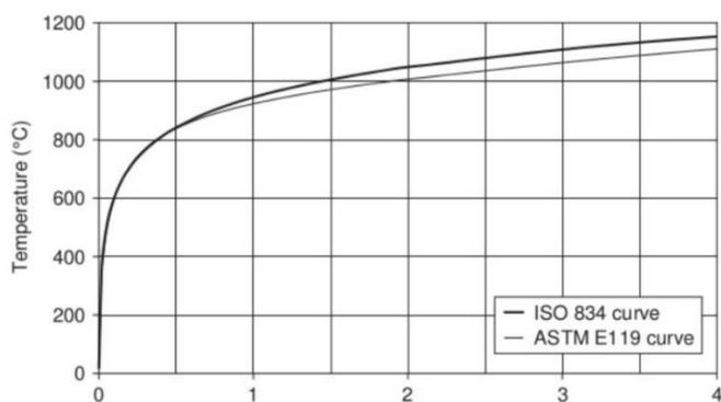
*Figure 3. Comparison of Standard Temperature-Time Curves [8]*
