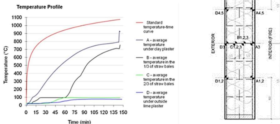
Figure 8. Temperatures in the wall during the test and cross section of the wall [16]
