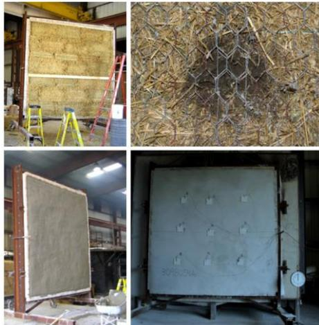
Figure 4. Preparation of the straw bale wall test specimen [9]
