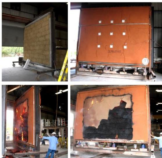
Figure 7. Photos before and after testing the specimen [10]
