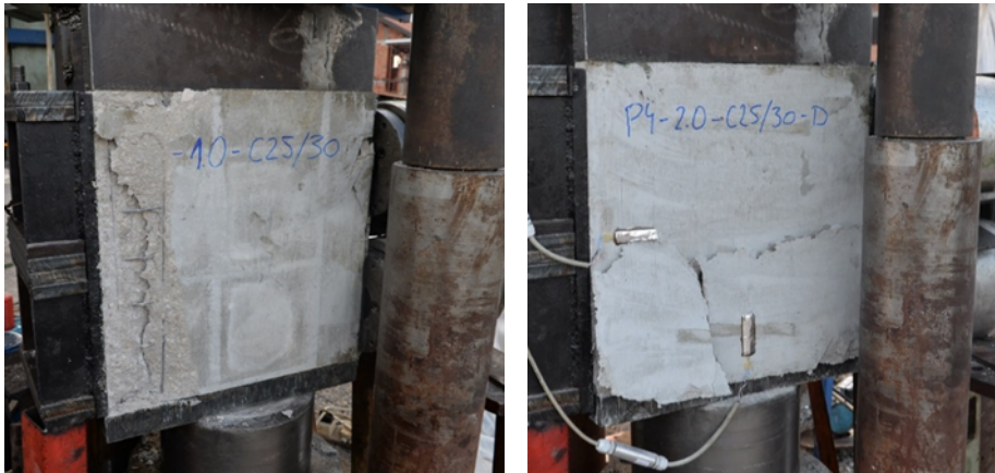
Figure 5: Failure of concrete panel (stress ratio 1.08 left) / (stress ratio 0,57 right)
