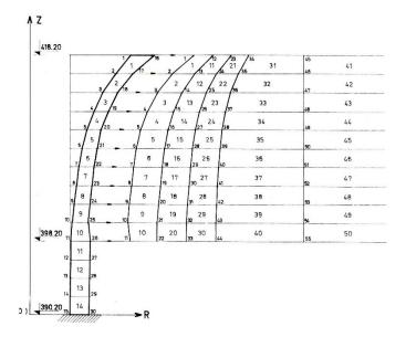
Figure 3. Mesh for FE and BE
