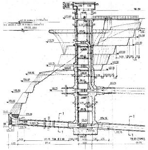
Figure 2. Water intake tower
