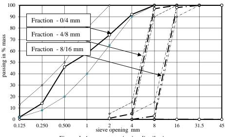
Figure 1. Aggregate grain size distribution
